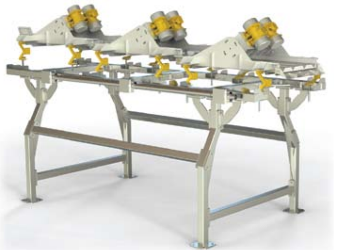
Aligning frozen meat pieces using vibratory feeders
