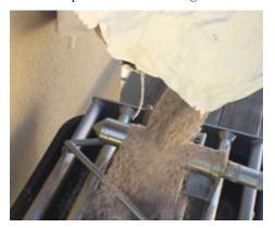
Picture 1: Testing individual ingredients on a bag opening grid.
