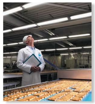
Poor lighting design can lead to uncleanable surfaces. pest harbourages and debris falling into food products.
